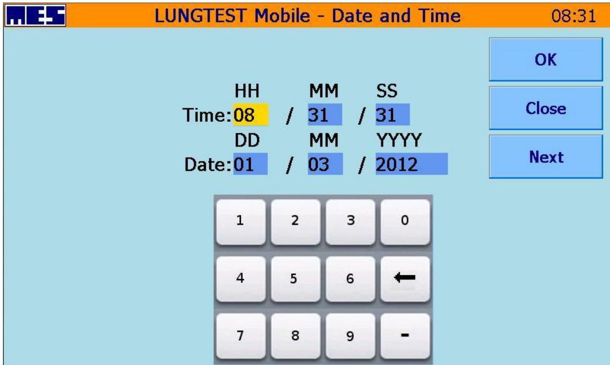
Fig 47 The “Date and Time” screen used to change the date and time on the spirometer
