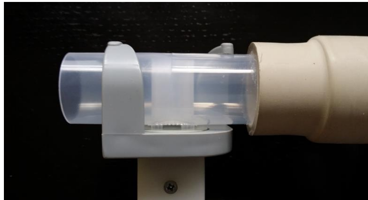
5.2b. Headpiece connected to the air-tube
