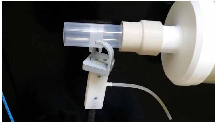
5.2a. Plugging the headpiece to the air-tube connection
