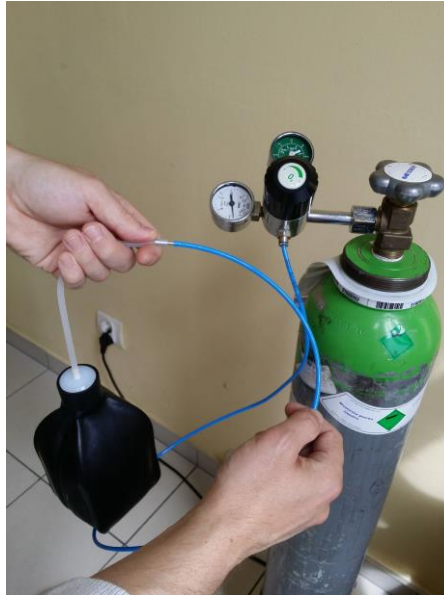
5.3b. Filling the calibration bag with gas
