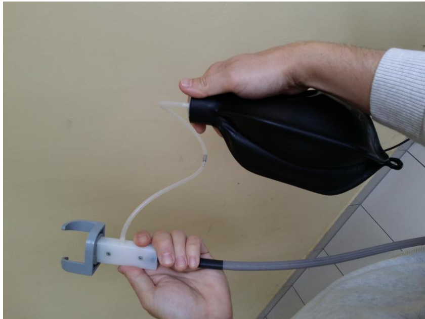
5.3c. Connecting the calibration bag to the air-tube
