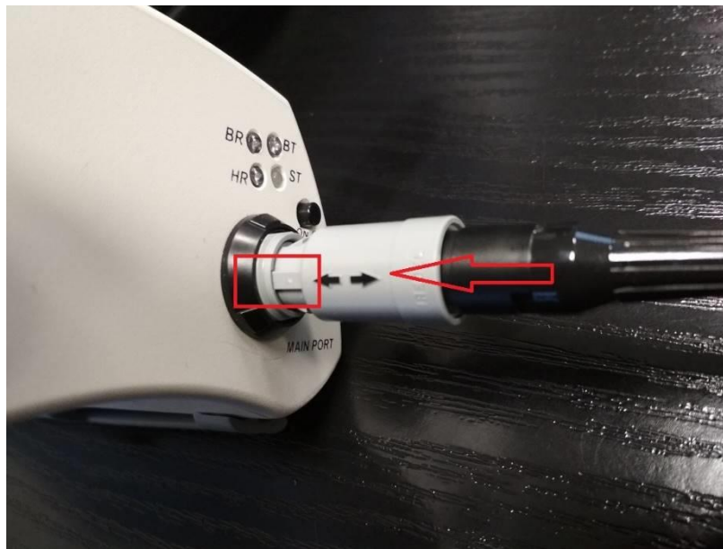
Fig 3d: Connecting the cable
