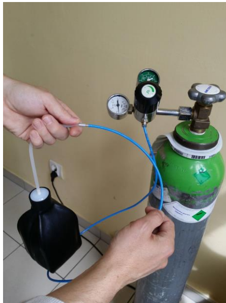
6b. Filling the calibration bag with gas
